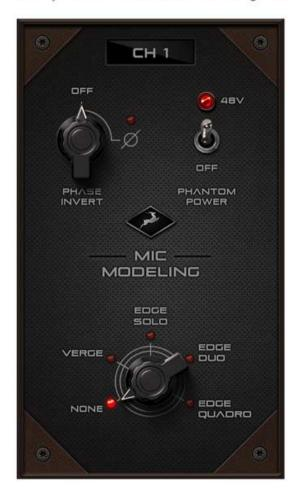
Note: 48V Phantom power will be automatically enabled.
