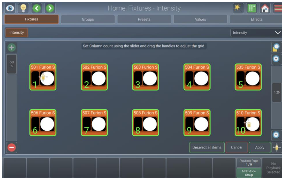
Fig. 96: Fixture View – Arrange Grid
