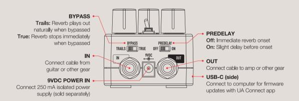
Power Supply Isolated 9VDC, center-negative, 250 mA minimum,
