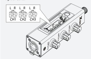
6. Wearing earphones/headphones, turn on the power and slowly adjust the PX-A master volume to the appropriate level. Then, adjust the volume of each channel at the source/s (e.g. aux output levels on the soundboard) to achieve a good starting mix. During performance, adjust channel volumes and master volume on the PX-A as needed.
