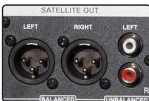
These jacks should be connected to the inputs of your active studio monitors or the inputs of a power amp that drives passive monitors. The signal is simultaneously available from all connectors.
