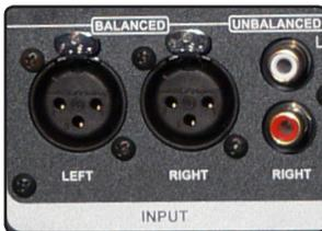
These stereo jacks - XLR in the balanced (also named: symmetrical), Cinch or RCA in the unbalanced (also named: asymmetrical) case, should be connected to the output of your mixing console or stereo/surround sound system.
