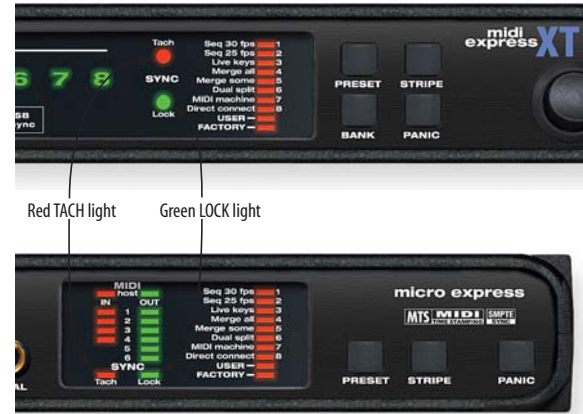
Figure 7-2: Converting time code. When your Express interface converts incoming time code, the red TACH light blinks, the green LOCK light glows steadily, and the green Computer I/O light glows steadily as well.
