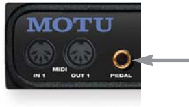
Figure 2-7: Connecting a foot switch or foot pedal.
